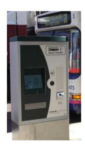
Norfolk County Council have introduced fourteen brand new state-of-the-art touch screen Ticket Vending Machines (TVMs) at key locations throughout Norwich to improve the efficiency of bus services by reducing the time taken to pick up passengers at busy bus stops.
